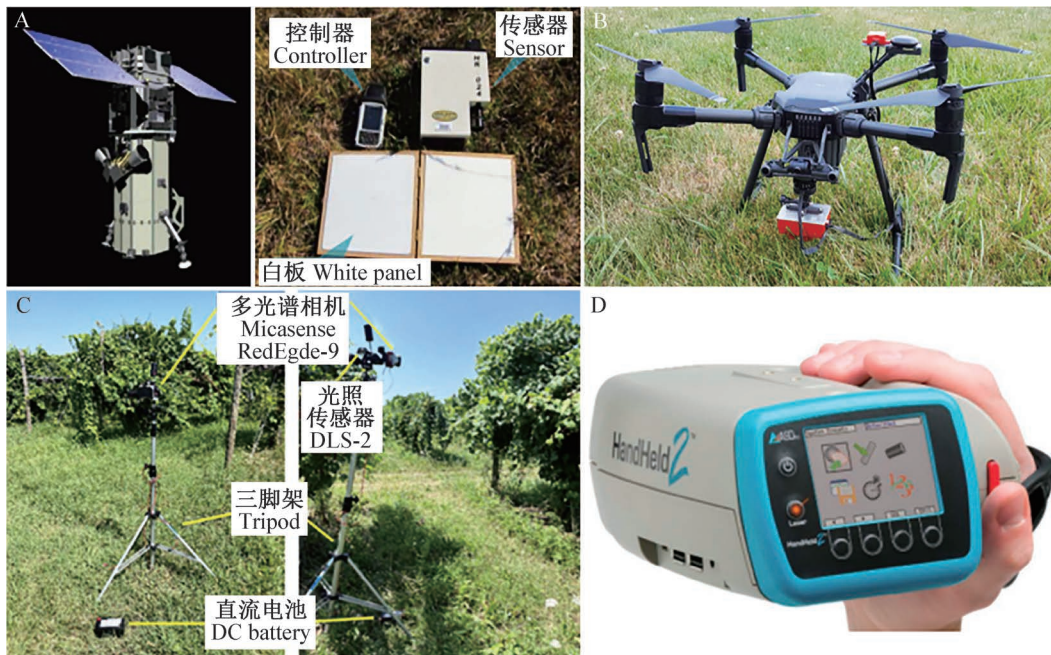
A: 遥感卫星多光谱传感(Bagheri, 2020); B: 无人机多光谱传感(Xiao et al., 2022); C: 地面多光谱传感(Saccuti et al., 2025); D: 小型手持多光谱传感(Wikantika et al., 2023)。A: Satellite-based multispectral remote sensing (Bagheri, 2020); B: UAV-mounted multispectral sensing (Xiao et al., 2022); C: ground-based multispectral sensing (Saccuti et al., 2025); D: portable handheld multispectral sensing (Wikantika et al., 2023)。
