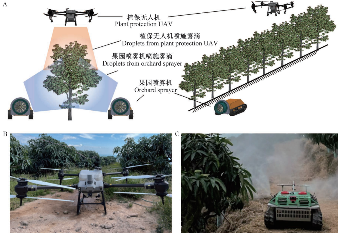
A: 果园空-地协同立体施药示意图; B: 空中施药装备; C: 地面施药装备。A: Schematic diagram of air-ground cooperative stereo pesticide application in orchards; B: aerial pesticide application equipment; C: ground pesticide application equipment.
